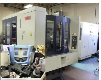
Baum Precision and our customers the ability to have up to 35 different jobs set up simultaneously. This greatly improves our set-up time by up to 80 percent through "externalizing" the tool and fixture set ups from the machining operation.
